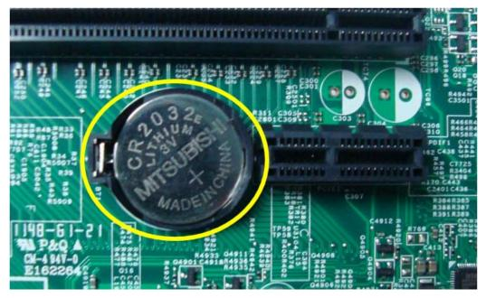
Note:RTC battery has been highlighted with the yellow circle as above image shows.Please detach the RTC
